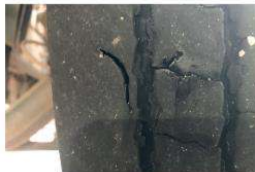
Tyre cut to cords
