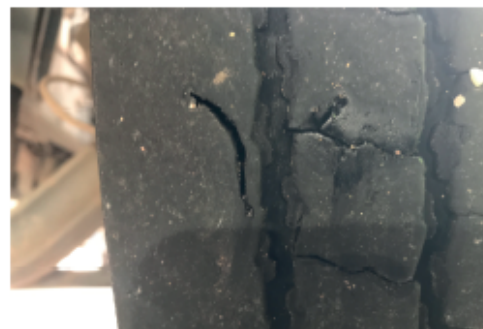
Tyre cut to cords
